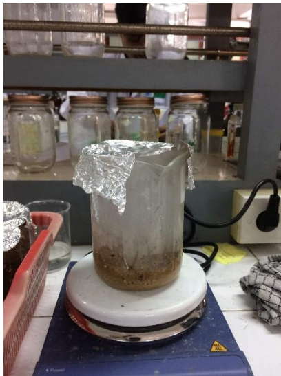
Proses Wet Peroxide Oxidation
