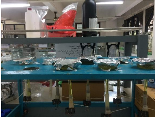
Proses Density Separation
