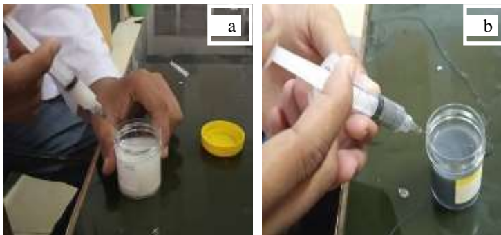
Gambar 4.5 Injectable Performance (a) Biokomposit Alginat/PVA; (b) Biokomposit Alginat/PVA/rGO
