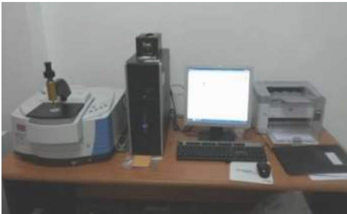
Gambar 3.7 Alat Uji FTIR
