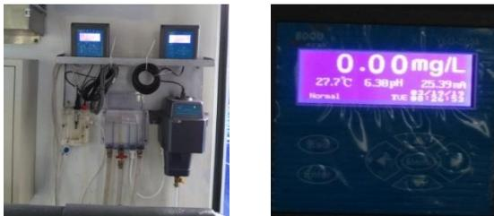
Gambar 5. 39 *Residual Chlorine Monitor*
