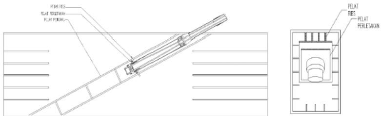
Gambar 4. 55 Plat angkur tendon
