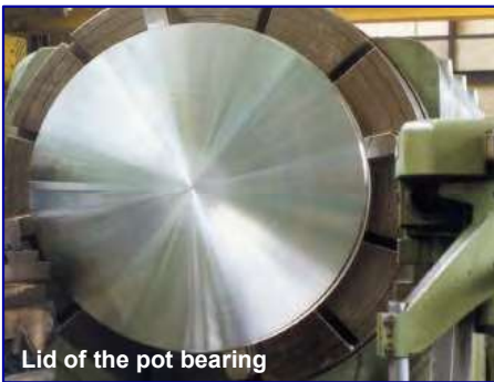
Formation of a steel ring
