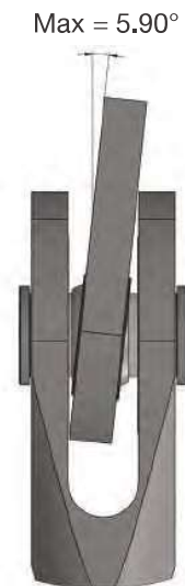
Additional misalignment with spherical bearing
