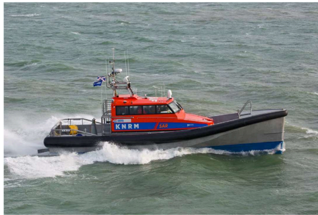
Gambar II. 12 Kapal self-righting rescue boat Damen (Sumber: Product Sheet Damen Search and Rescue 1906)
