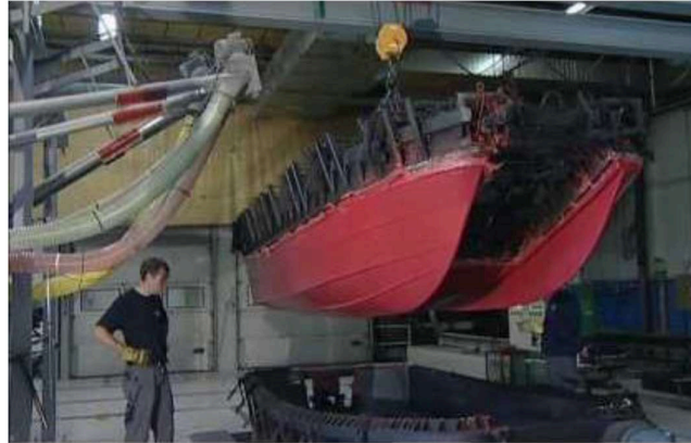
Gambar II. 18 Proses rotating molding kapal HDPE
