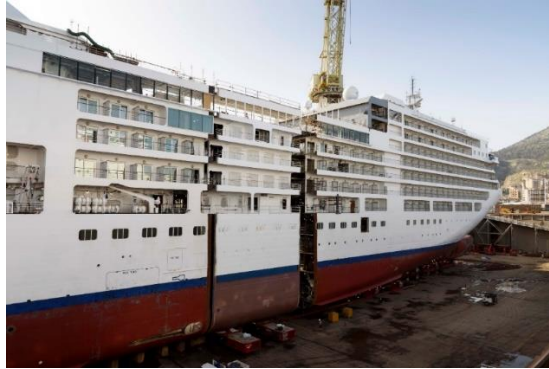
Gambar II.8 Modifikasi Insert hull Kapal Silver Spirit (sumber : www.maritime-executive.com )
