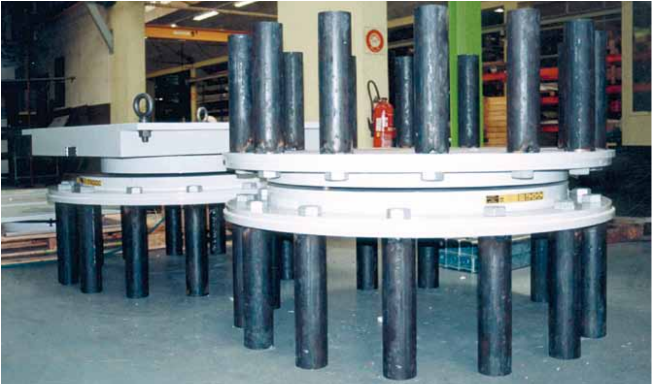
C380 Viaduct – Taiwan: pot bearings for very high horizontal seismic loads
