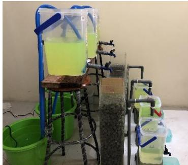
**Gambar 4.14 Color Tracer Test**
