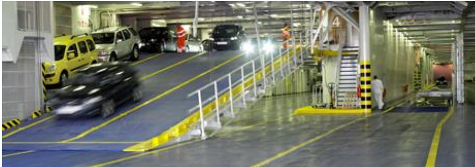
Gambar II.2 Internal Access Ramp
