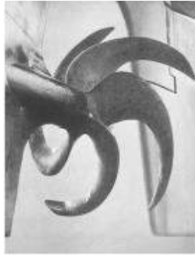
(e) biased high-skew, low-blade-area ratio propeller
