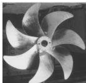
(c) FPP dengan 7 daun propeller blanced high-screw design
