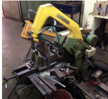
Gambar III.8 Proses Pemotongan Test Coupon
