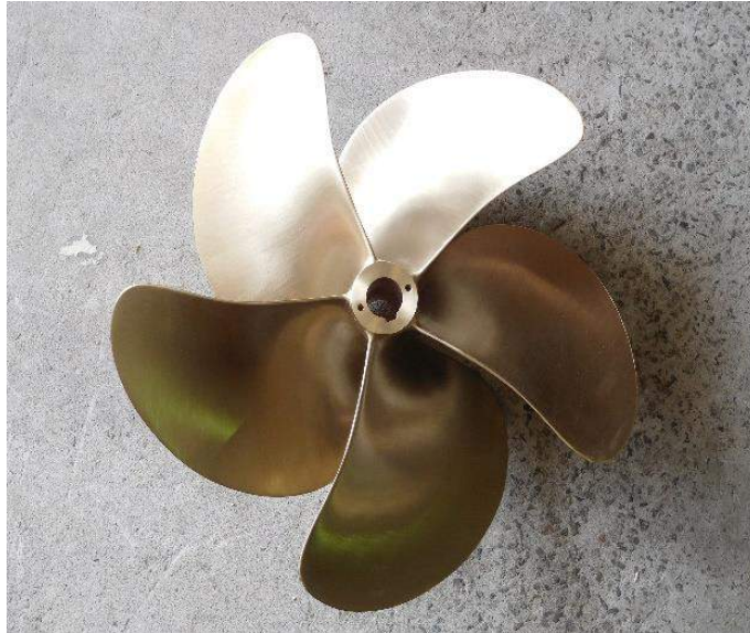
Gambar III.8. Propeller 5 blades (Sumber: https://www.mjengineering.com.au )
