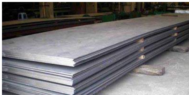
Gambar III.7. Material JIS G3101 SS400 (Sumber: http://www.steel-plate-china.com )
