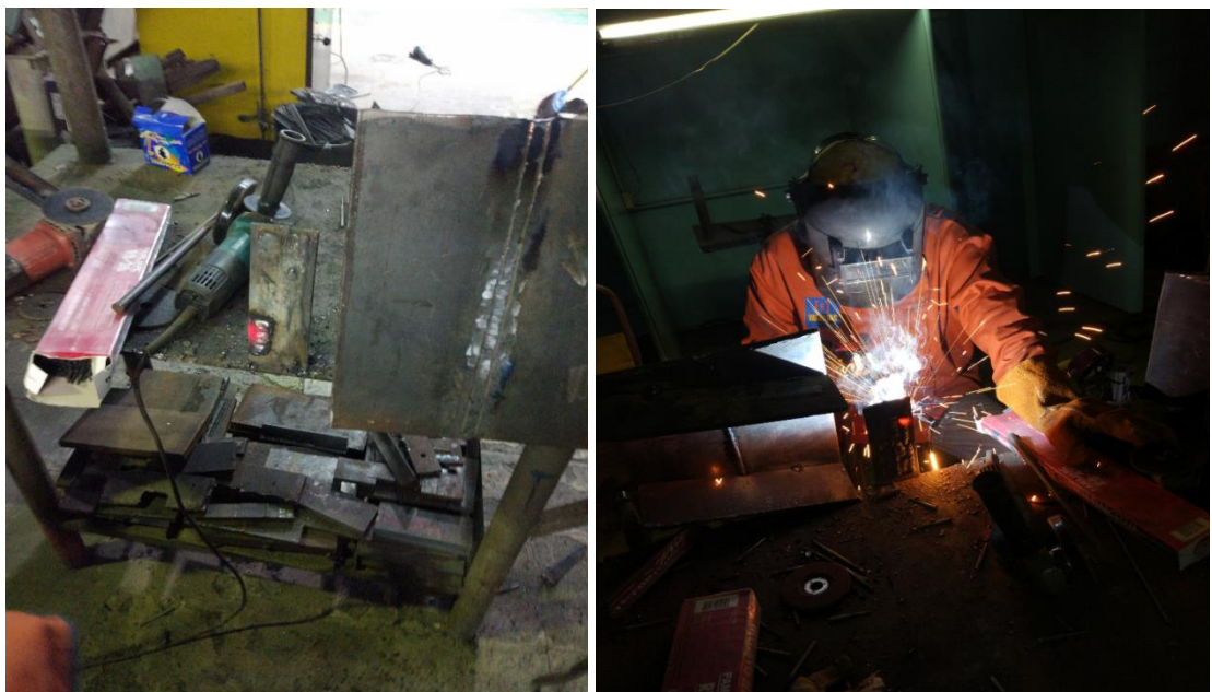
Gambar III.14 Demo Heat input Temper Bead Welding
