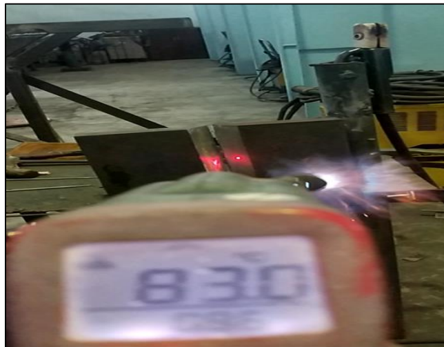
Gambar III.10 Preheat di atas 60°C
