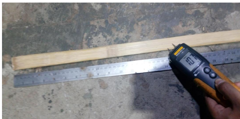
Gambar 3.3 Proses Pengukuran Kadar Air
