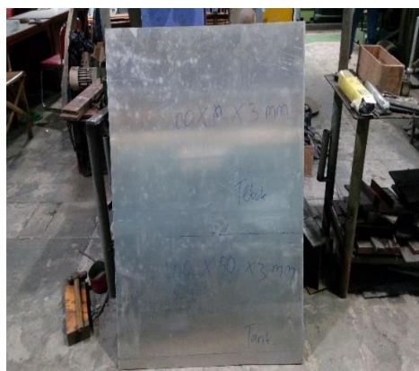
Gambar 3.7 Aluminium Marine Use Tipe 5083
