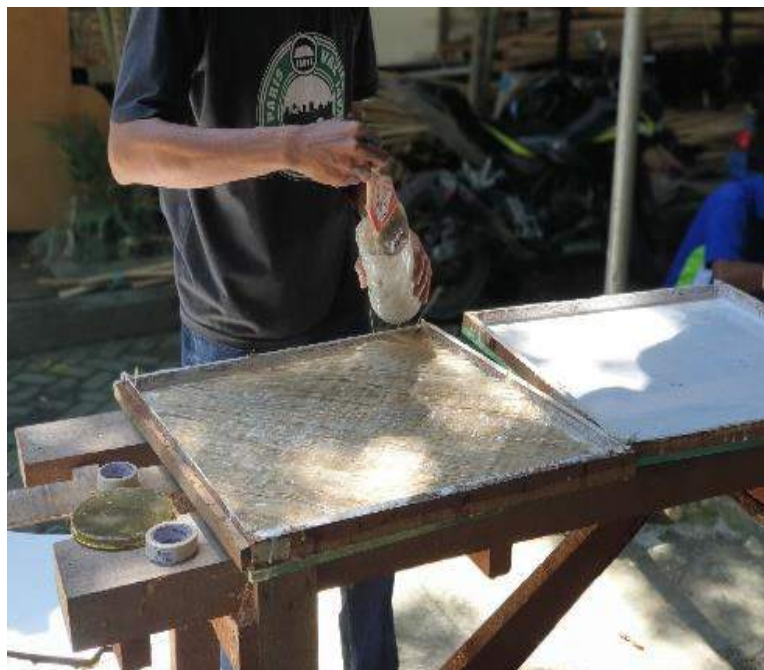
Gambar 3.14 Proses laminasi CSM 300
