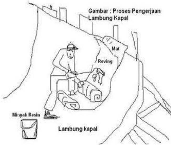
Gambar 2.15 Proses laminasi [sumber: Ardiana, Razali, Muharnis, 2014]
