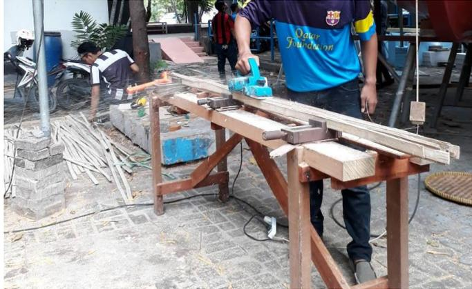
Gambar 3.6 Proses *finishing* gading
