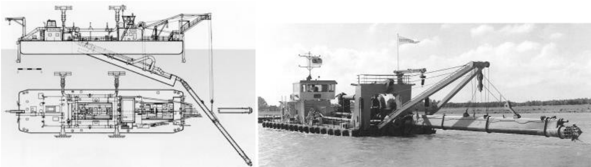
Gambar II. 8. Plain Suction Dredger (W.J. Vlasblom, 2003)
