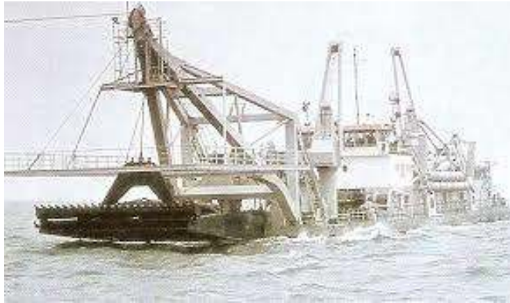
Gambar II. 7. Dustpan Dredger (Dredge Point, 2016)
