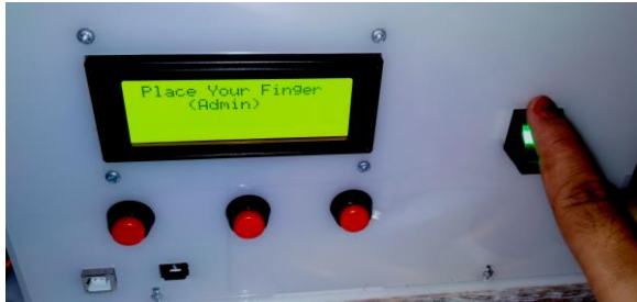
Gambar 4.16 Proses Admin Scanning Sidik Jari
