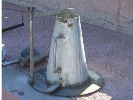
Gambar 4. 22 Kerucut uji slump
