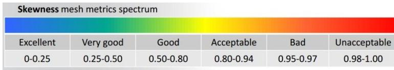
**Gambar 3.8** Mesh metric spectrum
