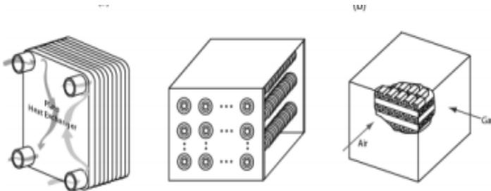
**Gambar 2.1** (a) brazed plate heat exchanger (b) circular-finned tube heat exchange (c) plate fin heat exchanger (Incropera, Dewitt, Bergman, & Lavine, 2011).
