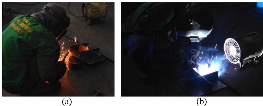
**Gambar 3.15** (a) Proses *Tack Welding*; (b) Proses Pengelasan
