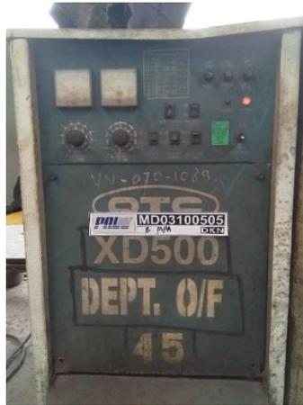
**Gambar 3.2** Mesin FCAW (*Flux Core Arc Welding*)
