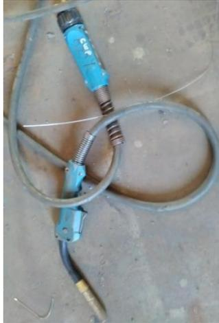
**Gambar 3.4** FCAW Welding Gun
