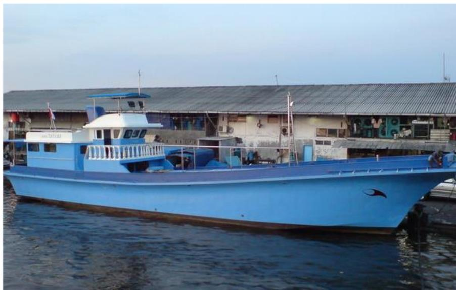
**Gambar 2.28.** Kapal *Pole and line* 57 GT (Wahana Fiberglass, 2019)
