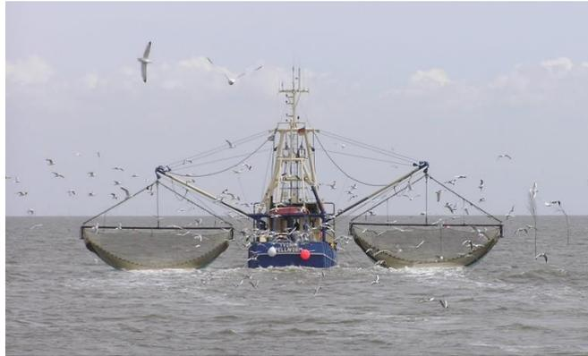
**Gambar 2.9.** *Liftnet* (Wikipedia, Fishing vessel)
