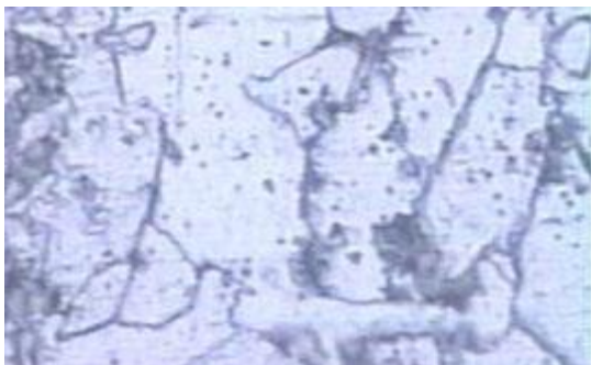
(c) Weld Metal
