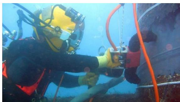
Gambar 4. 21 Magnetic Particle – Underwater Inspection
