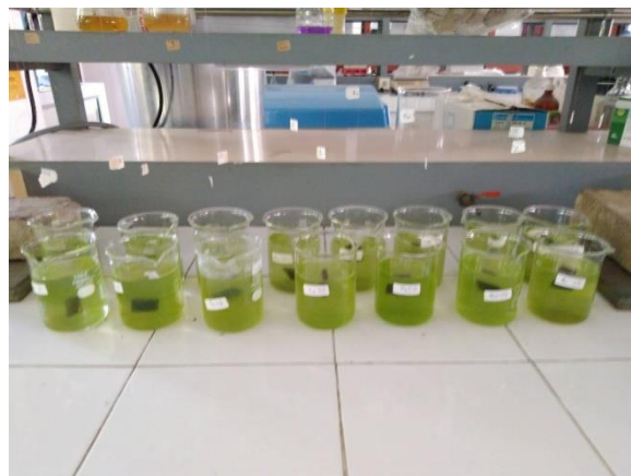
Gambar 4. 12 Proses Pengujian Immersion Corrosion Test
