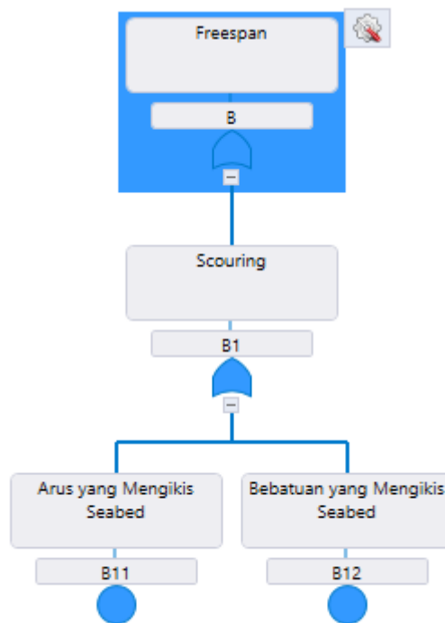
Gambar 4.4. Diagram Fault Tree Analysis Freespan
