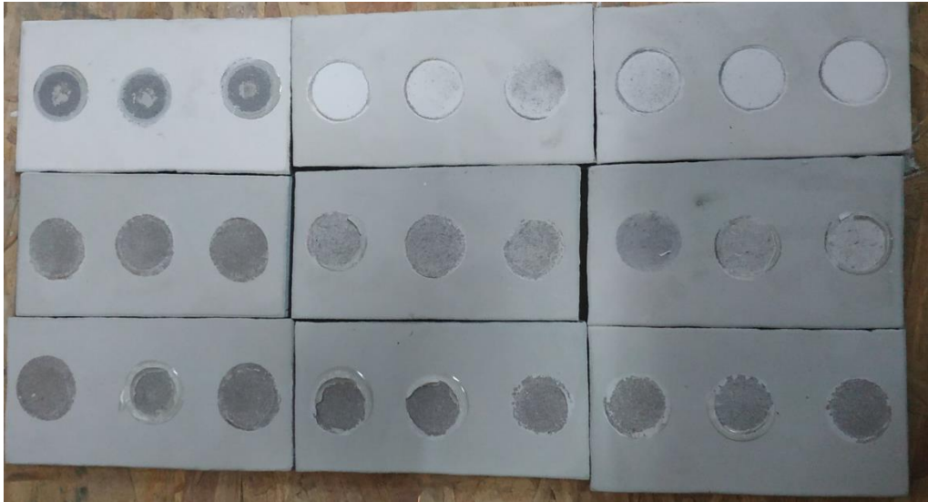
Gambar 4.6. Hasil Pull Off Material
