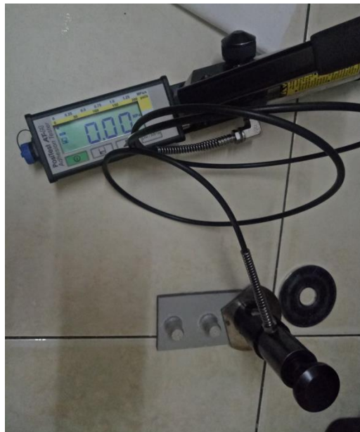
Gambar 3.13 Portable adhesive tester
