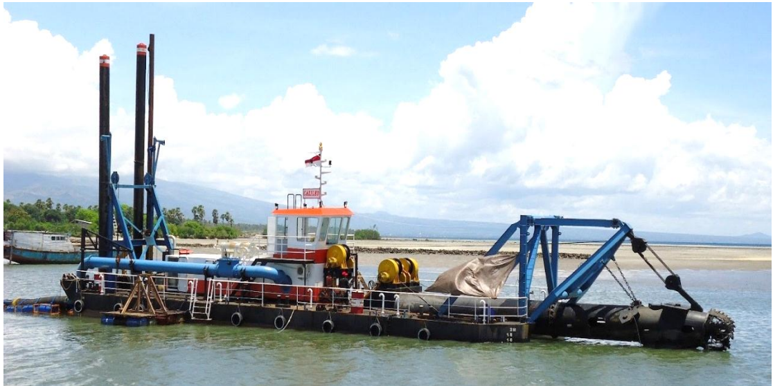
Gambar 2.1 Cutter Suction Dredger (sumber : cahayamentaricemerlang.blogspot.com)
