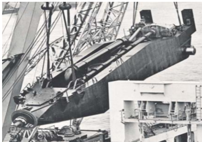
Gambar 2.4 Cutter Head Ladder (sumber : Vlasblom, 2005)
