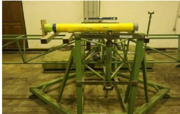
Gambar 3.7 Kalibrasi Centre of Gravity (CoG)
