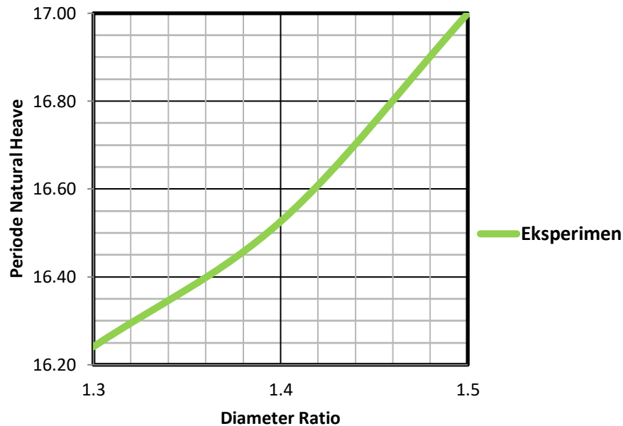
Gambar 4.11 Grafik Fungsi Diameter Ratio Terhadap Periode Natural Heave Classic SPAR + Heave Plate
