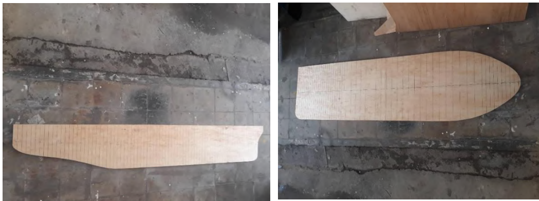
Gambar III.6 Sheer Plan Profile dan Half Breadth Profile
