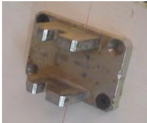
Gambar III.15 Holder poros pengarah
