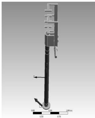
Gambar 4.5. Arah Pembebanan *Frame* Poros Dari  $225^{\circ}$
