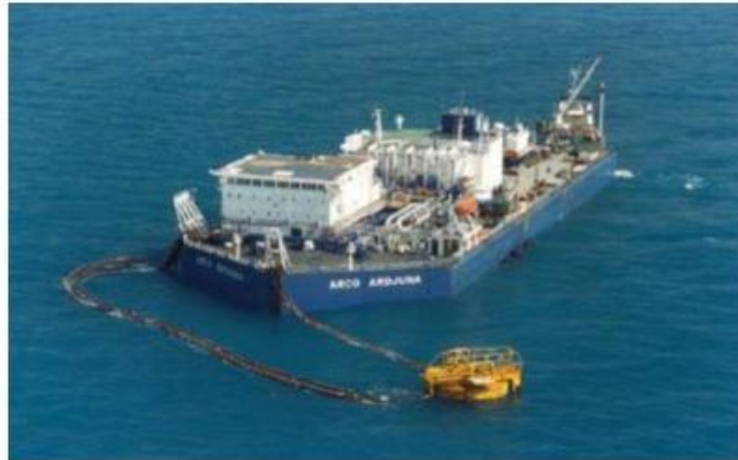
Gambar 2.4 Catenary Anchor Leg Mooring (CALM) buoy (Sumber: PT. PHE ONWJ, 2013)
