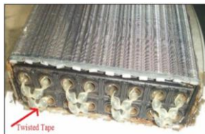
Gambar 2. 3 Aplikasi Twisted tape insert (a) radiator mobil (Hasanpour, Farhadi, & Sedighi, 2014) (b) shell and tube heat exchanger (Koch Heat Transfer, 2018)
