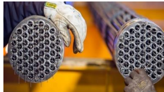
Gambar 2. 3 Aplikasi Twisted tape insert (a) radiator mobil (Hasanpour, Farhadi, & Sedighi, 2014) (b) shell and tube heat exchanger (Koch Heat Transfer, 2018)
