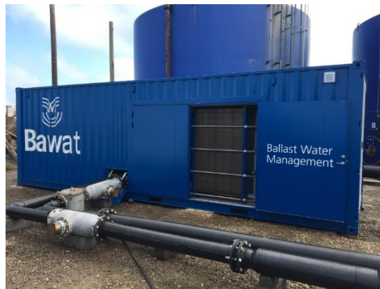
Gambar 2. 6 Land-based Ballast Water Treatment (Sumber : www.ballastwatermanagement.co.uk )
