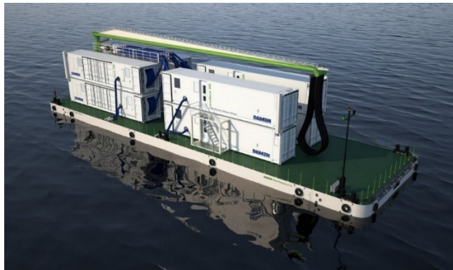
Gambar 2. 7 Barge-Based Ballast Water Treatment (Sumber : Damen Green, 2018)
