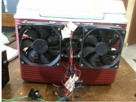
**Gambar 2. 13 Thermoelectric Cooler Box**
