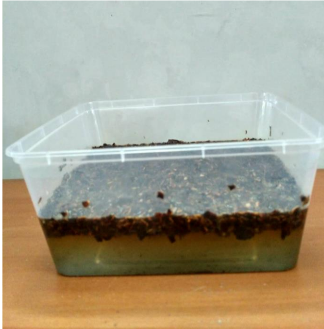
Proses Perendaman Alkali NaOH
