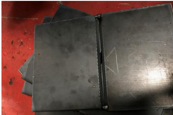
Gambar 3.2 Material Baja ASTM A53 Grade B
