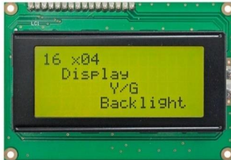
Gambar 2. 10 LCD 16 x 4 Sumber: Winstar Display
