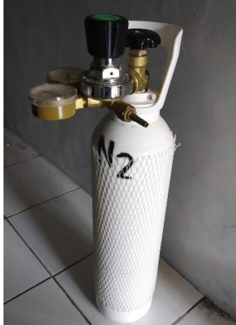
Gambar 3. 13 Tabung Gas Nitrogen
