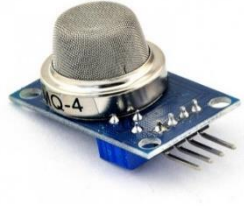
Gambar 2. 5 Sensor MQ-4 Sumber: Datasheet MQ-4
