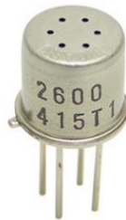
Gambar 2. 7 Sensor TGS2600 Sumber: Datasheet TGS2600
