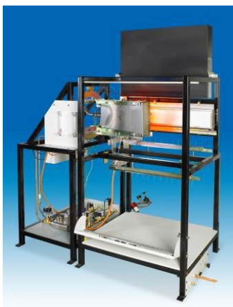
Gambar 2.6 Flame Spread Apparatus (Sumber: fire-testing.com )
