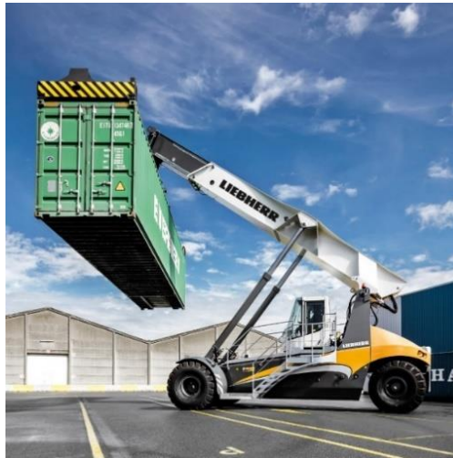
Figure 2.9. Reach Stacker Source: Property of Liebherr
