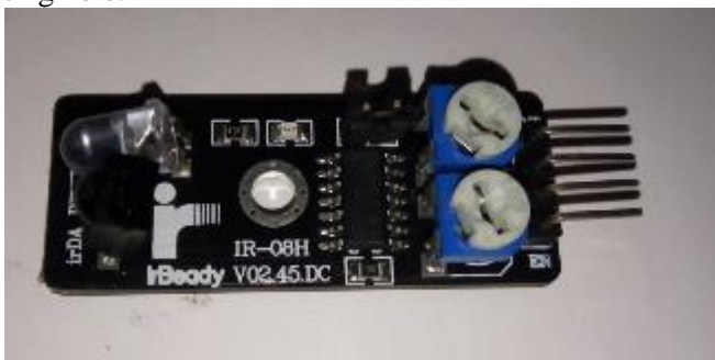
Gambar 2. 4. Hardware Detail IR Proximity Sensor Sumber : (Silicon TechnoLabs, 2015)
