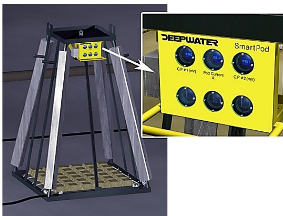
Gambar 2.5. Desain anoda Deep Water Monitored Anode Pod Array
