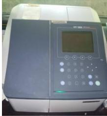
**Gambar 2. 11** Spektrofotometer UV-Vis *double-beam*
