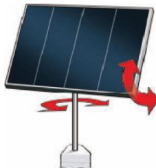
Gambar 2. 2 Dual axis solar tracker
