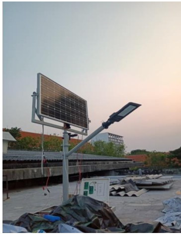
Gambar 3. 18 Prototype active solar tracker
