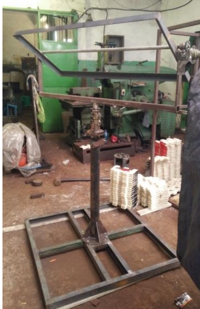
Gambar 3. 4 Realisasi subsistem mekanik solar tracker
