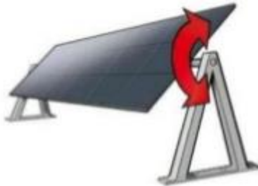
Gambar 2. 8 Single Axis Tracker[17]
