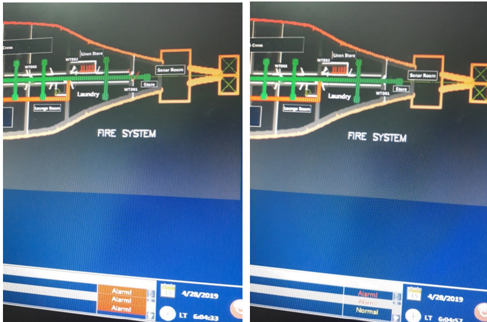
Fig. 4.10. Reaction of Notification While Open and Close Watertight Door Occurs in the MIMIC Display
