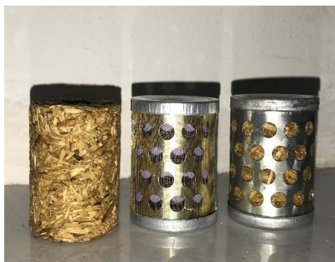
Figure 3.6 Modified Sawdust Oil Filter Final Product
