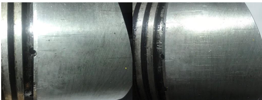
Figure 4.9 MSF Equipped Engine Piston (left), CMF Equipped Engine Piston (right)
