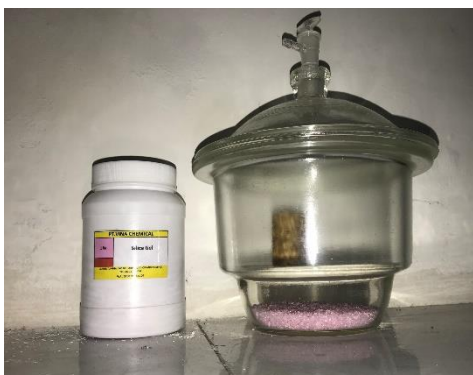
Figure 3.5 Desiccator for Modified Sawdust Cooling Process
