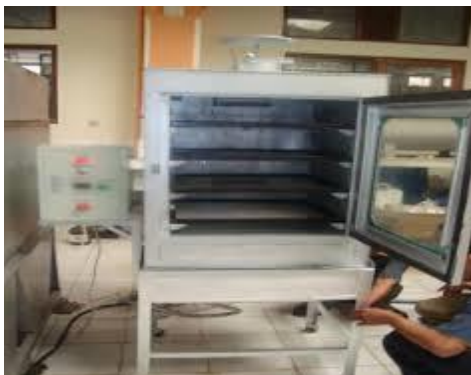
Figure 3.4 Dry Oven for Modified Sawdust Drying Process
