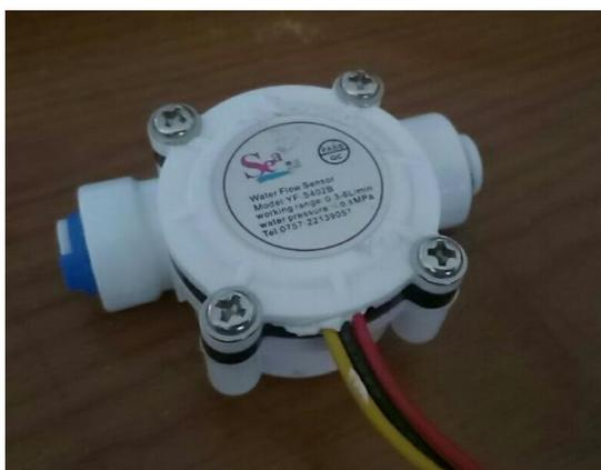
Gambar 3.6 Flowmeter Sensor YF-S402B
