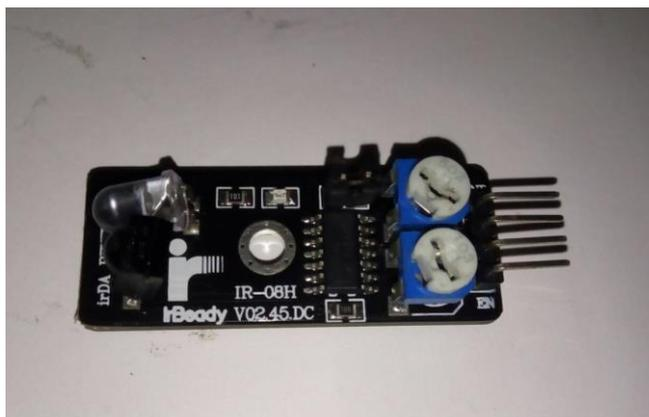
Gambar 3.11 RPM Sensor IR-08H
