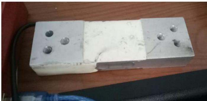
Gambar 3.8 Load Cell 100 kg
