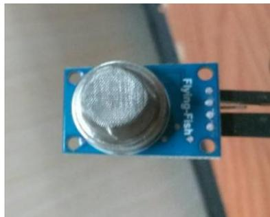
Gambar 3.2. Modul Sensor MQ-135
